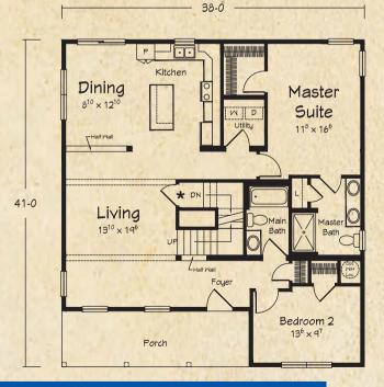
For elevated piling/pier foundations, a site built enclosed entry from grade level can be built at stair areas showing \* symbol.
